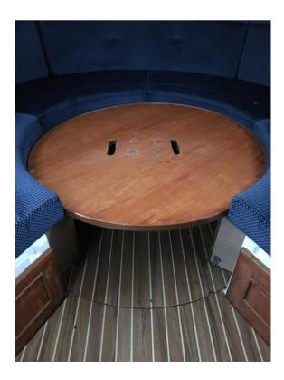
Lift flooring panel up from step and place at foot of the table,
