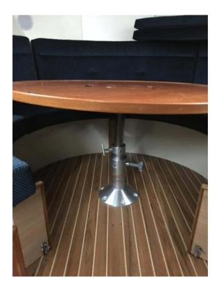
Using the screws on the leg of the table, lower it until it sits level with the base of the seating (as seen below)
